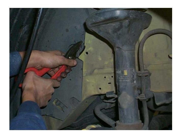
10. Now remove the cross bars from the lower brackets, line up the brackets, and have the other person line up the "L" backing plate. This backing plate will cover the holes in the actual strut tower for the bracket. You line it up from inside the wheel well. Put the bolts in, you may notice a little difficulty doing this, at least we did, what we did to solve it, is use the slightly larger drill bit and bore out the holes just a little more that we made on the body panels.
